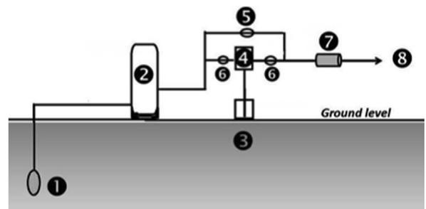
**Fig. 1.** Schematic view of the farm's water distribution system. 1: Borehole pump, 2: water buffering tank, 3: Dinastim™ or Pigfast™ delivery tank, 4: dosing distribution pump, 5: bypass, 6: pumps, 7: position of experimental coupons, and 8: to the troughs.
