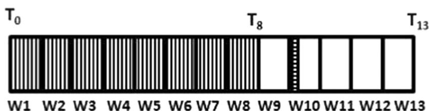
**Fig. 2.** Time sequence for the treatment of drinking water distribution systems. Units are weeks. Dinamycol™ (vertical hatching) is applied for eight weeks (W1 through W8), Pigfast™ (horizontal hatching) is applied for two days at the beginning of week ten (W10). Biofilm observations were made at T<sub>0</sub>, T<sub>8</sub> and T<sub>13</sub>.
