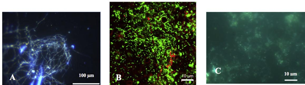
**Fig. 3.** Observations in confocal microscopy of the water pipe's inner surface (Breeding Unit A). A, T<sub>0</sub>, B, T<sub>8</sub>, C, and T<sub>13</sub>. A and C are labelled with DAPI, B is labelled with the Dead/Live kit so that living cells exhibit green fluorescence whereas dead ones appear red.
